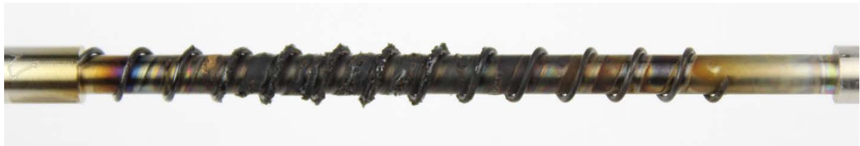
Figure 60: Synthetic oil #4 TEOST MHT rod deposits
