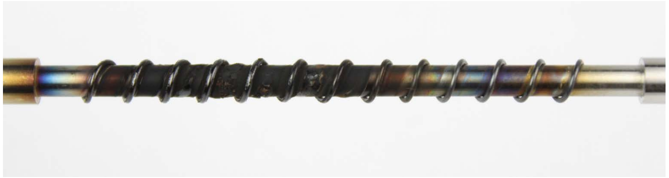
Figure 54: Synthetic oil #1 TEOST MHT rod deposits
