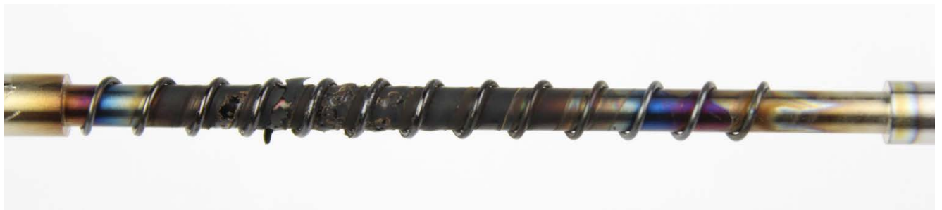
Figure 58: Synthetic oil #3 TEOST MHT rod deposits
