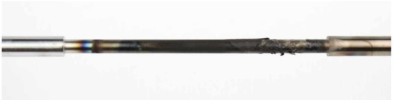
Figure 55: Synthetic oil #1 TEOST 33C rod deposits
