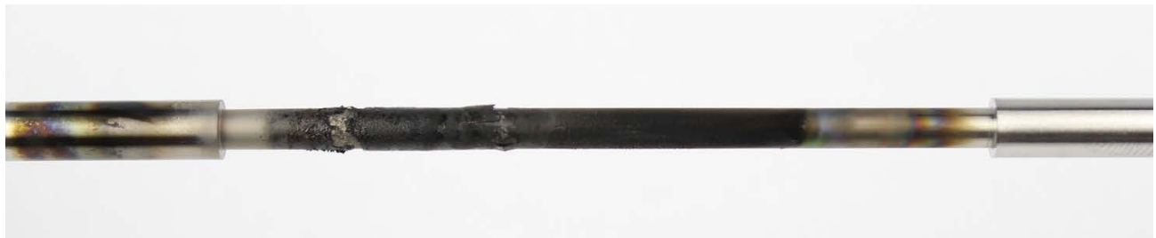
Figure 45: Conventional oil #1 TEOST 33C rod deposits
