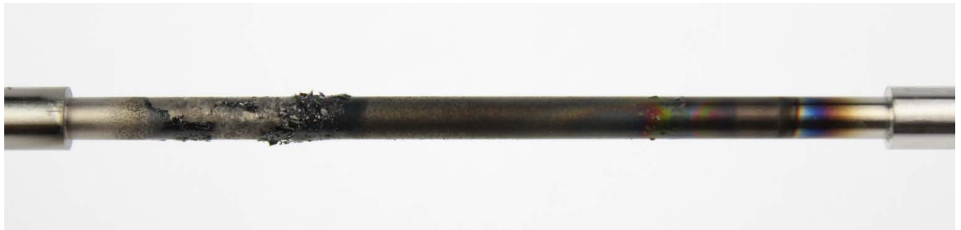
Figure 59: Synthetic oil #3 TEOST 33C rod deposits
