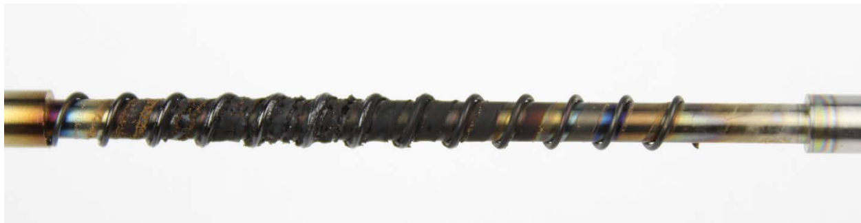
Figure 62: Synthetic oil #5 TEOST MHT rod deposits
