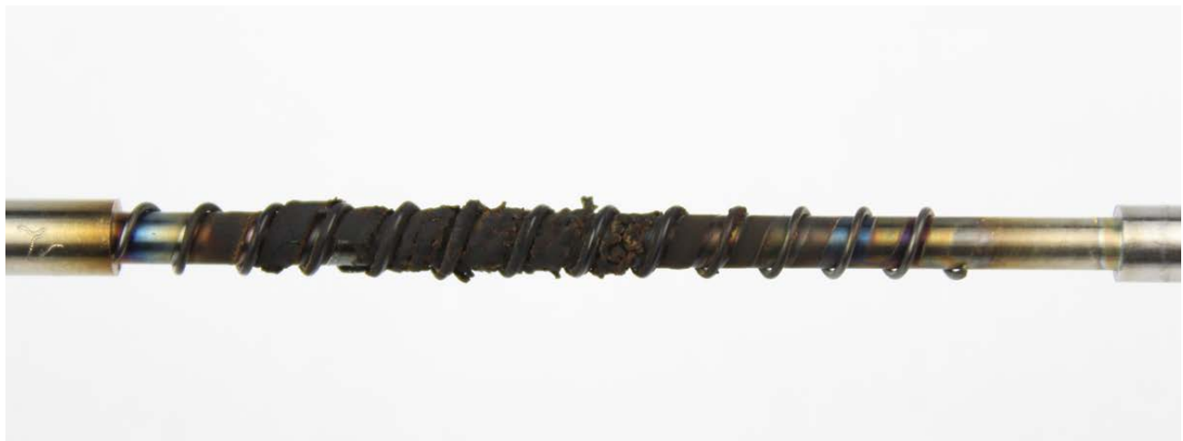
Figure 46: Conventional oil #2 TEOST MHT rod deposits
