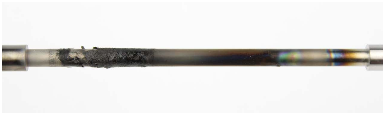
Figure 51: Conventional oil #4 TEOST 33C rod deposits
