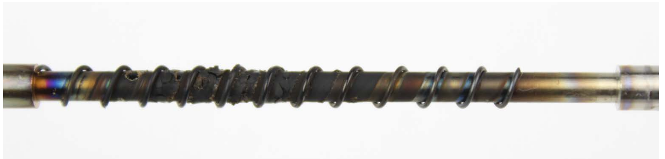
Figure 56: Synthetic oil #2 TEOST MHT rod deposits
