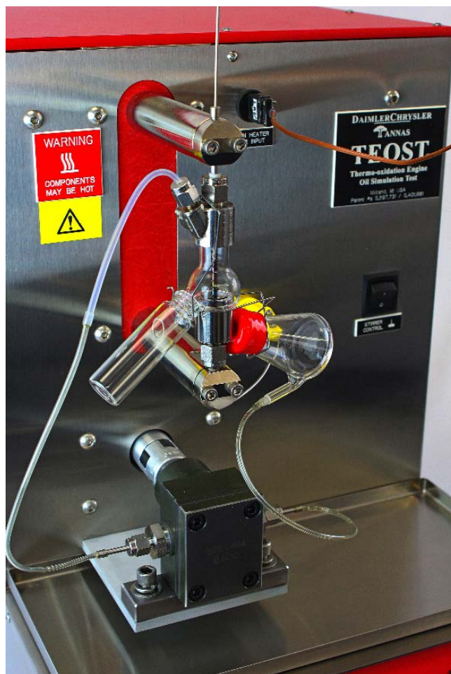
Figure 9: ASTM D7097 TEOST MHT instrument Image Source: AAA
