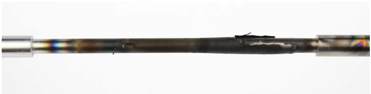
Figure 49: Conventional oil #3 TEOST 33C rod deposits
