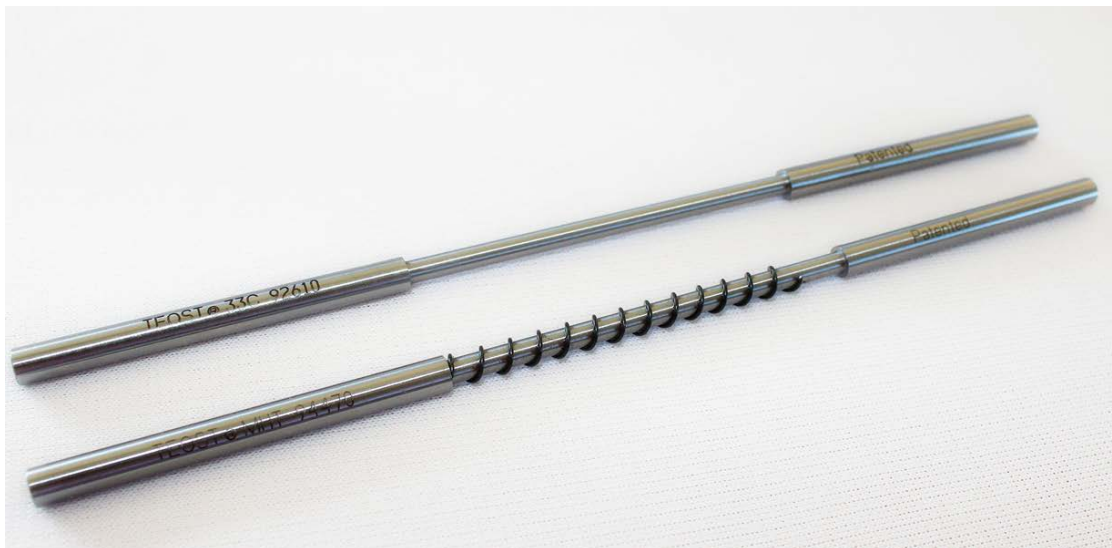
Figure 43: TEOST MHT & 33C depositor rods
