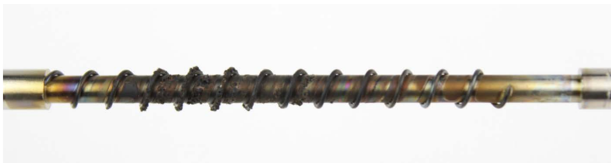
Figure 52: Conventional oil #5 TEOST MHT rod deposits
