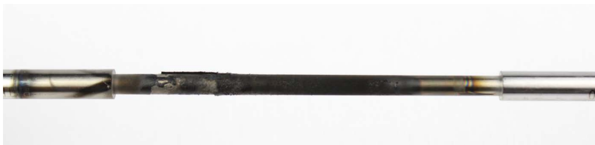
Figure 53: Conventional oil #5 TEOST 33C rod deposits
