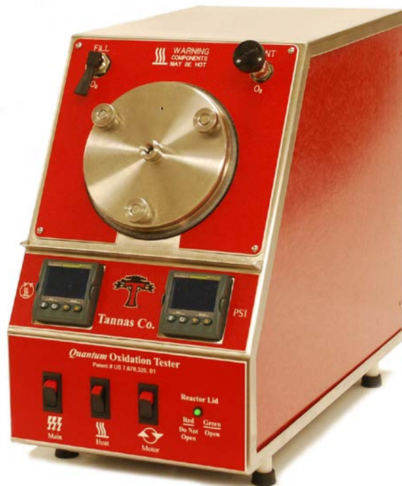
Figure 22: ASTM D4742 TFOUT instrument Image Source: AAA
