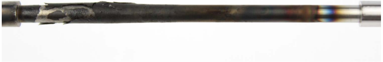
Figure 47: Conventional oil #2 TEOST 33C rod deposits
