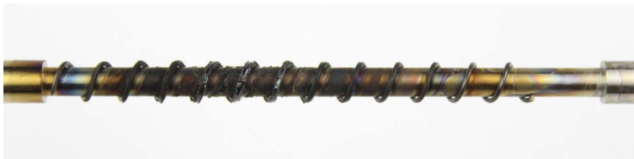
Figure 50: Conventional oil #4 TEOST MHT rod deposits
