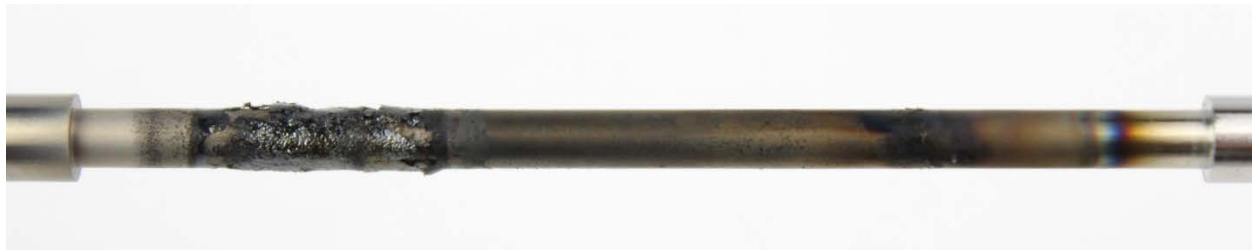
Figure 61: Synthetic oil #4 TEOST 33C rod deposits
