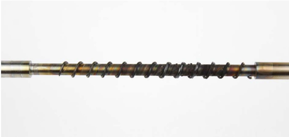
Figure 44: Conventional oil #1 TEOST MHT rod deposits
