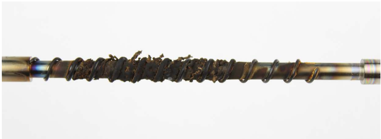
Figure 48: Conventional oil #3 TEOST MHT rod deposits
