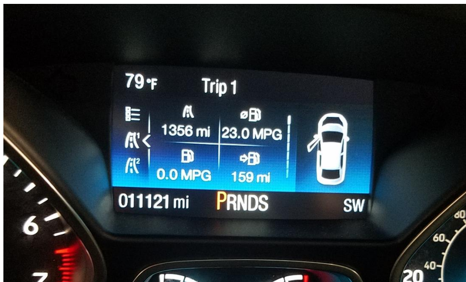
Figure 2: Example of fuel economy and range on vehicle display. Image source: AAA.
